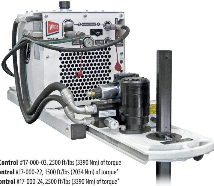
**HD Manual Control** #17-000-03, 2500 ft/lbs (3390 Nm) of torque
