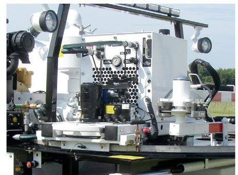
The TM-7 Swivel optional allows up to 15 degrees of valve stem misalignment
